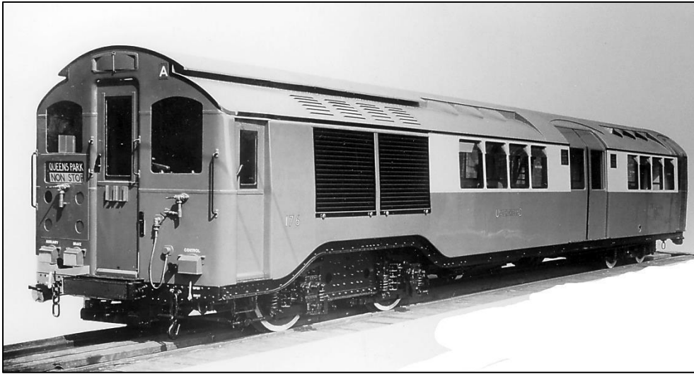
Figure 2: Watford Replacement Stock motor car at the Metro Cammell factory. It is not yet fully fitted out, for example, shoebeams are not fitted because they were likely to get damaged in transit between Birmingham and the Underground's delivery depot at Lillie Bridge. Photo: Official Metro Cammell.
