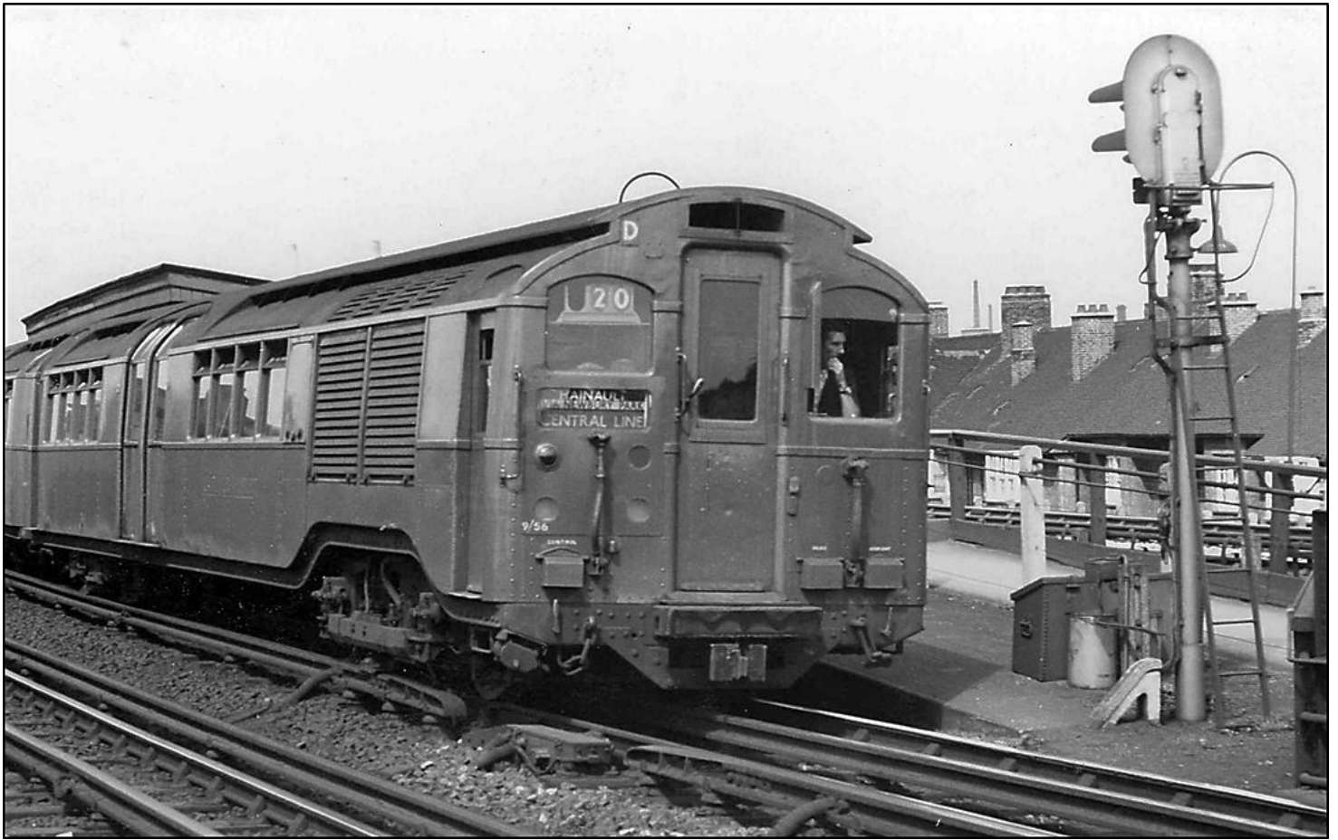
Figure 6: A 1924 Met. Carriage motor car leading a Central Line train at East Acton towards the end of its days. It shows an overhaul date of September 1956 and most of this type was withdrawn during 1961-62. The front of the train shows the near final state of the 1923-25 batch of cars with modified marker lights, new offside destination plate box, new set number location, ventilator added over the end door, a window wiper, e.p. brakes and relocated emergency lighting cable. Photo: Alan A. Jackson.
